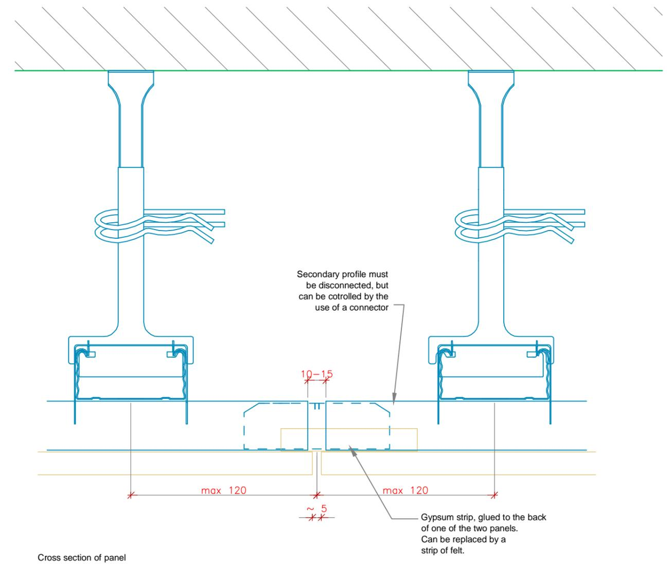
Where expansion joints are present in the primary constructions, the suspended ceiling construction must be correspondingly interrupted!
