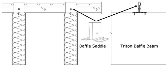
IFSS/IFSC internal fixing strip for screw fixing the Baffle to suspended frames such as Rondo Donn<sup>®</sup> grid with the Baffle Saddle (IFSS) or to furring channels (IFSC).
